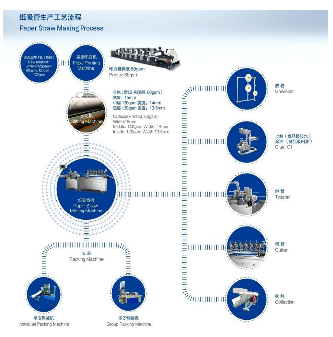
Note: The Flexo Printer is Optional. Smaller printer units are now available with most lines.
