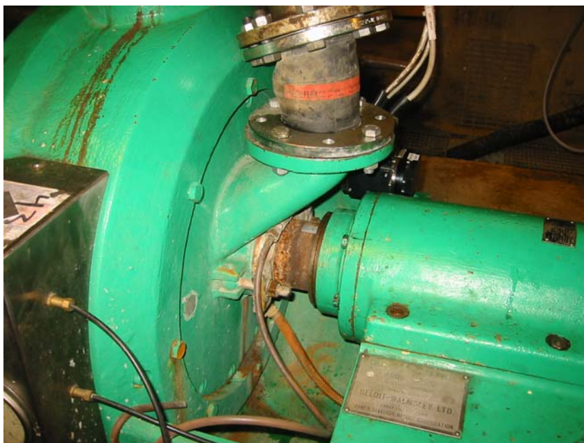
Figure 3.1. The photography shows the Beloit DD refiner seen from the fixed stator side. This stator door was replaced by another door incorporated the fibre-optic pressure sensors (Source: Ola Johansson, J&L Fiber Services Inc.).
