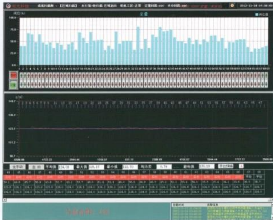
图二 横幅定量闭环控制后纸张横幅定量波动得到了根本的改善 cross direction basis weight fluctuation fundamentally improved after closed-loop control
