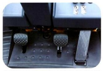
Optimized pedal position: The position of accelerator has been optimized through human engineering.
