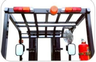
High strength mast and excellent visibility are desirable for safe operation. The panoramic mirror expands the driver's view when backing up.
