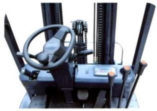
Our small diameter steering wheel features a standard spinner knob to maximize maneuverability and operator confidence.
