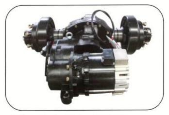
Water-resistant and dust-proof motor and controller: Provide excellent reliability even in wet weather.
