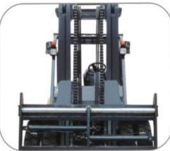
Heavy duty welded mast: Wide designed with good visibility, and ensures its excellent forward visibility, improves working efficiency and the safety.
